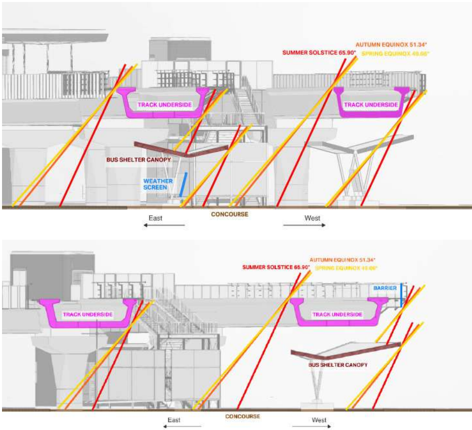
FIGURE 3-7 SUN ALTITUDE 2PM ON DOWN MAIN (TOP) AND UP MAIN (BOTTOM) BUS SHELTERS
