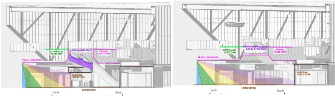
FIGURE 3-27 NORTHERN RAIN ANGLES ON NORTH (LEFT) AND SOUTH (RIGHT) STATION ENTRIES
