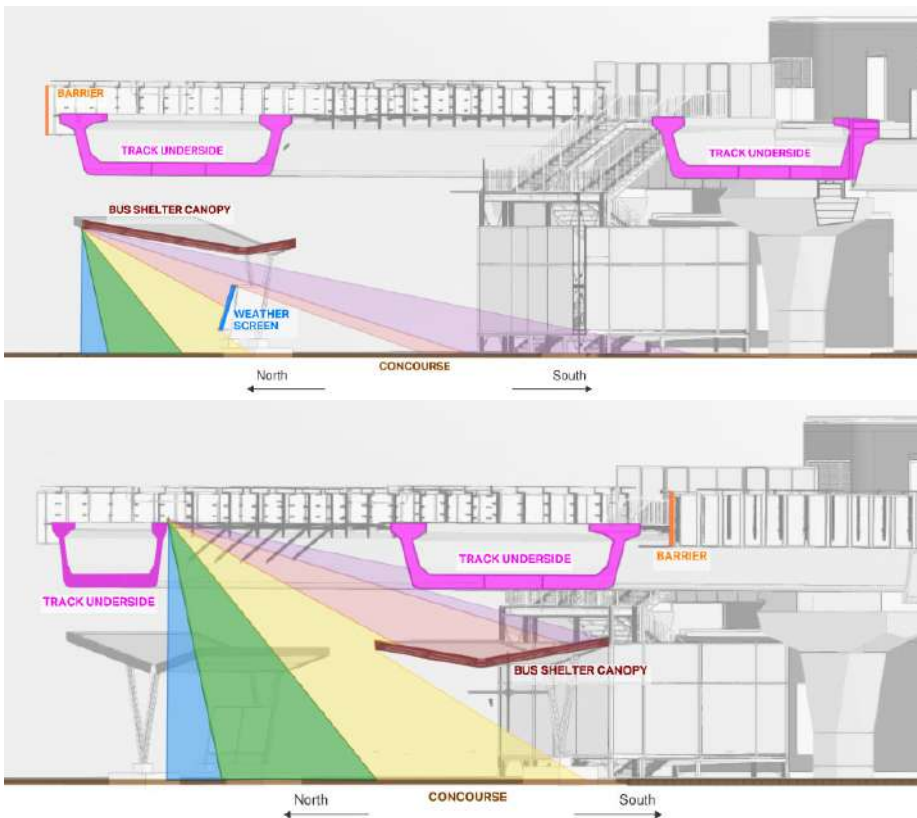
FIGURE 3-31 NORTHERN RAIN ANGLES ON BUS SHELTERS THROUGH DOWN MAIN (TOP) AND UP MAIN (BOTTOM) RAIL CORRIDORS
