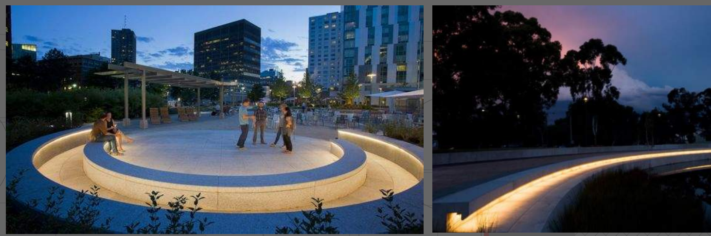
CIRCULAR SEAT ILLUMINATED WITH FLEXIBLE OUTDOOR LED NEON UNDER TOP MOST LIP PROVIDING SCULPTURAL AMBIENT GLOW TO SEATING AREA
