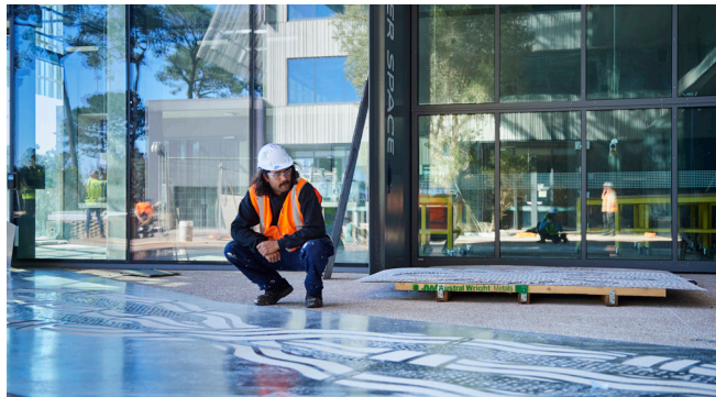
Judy Watson works with UAP pattern makers to ensure the weave is mounted onto foam correctly. These forms will be used in the sand casting process to make the moulds.
