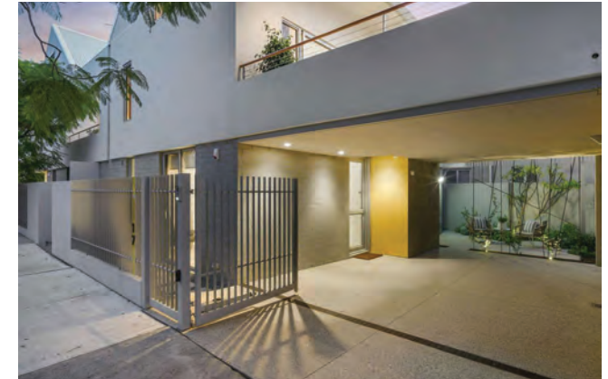
Photo G3.4a Undercroft parking reduces the visual impact of parking on the street and provides an opportunity for flexible use of the space when not required for car parking
