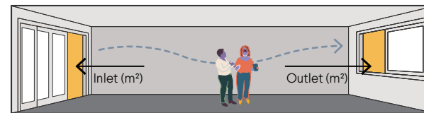
Figure G3.2b Natural ventilation for passive cooling
