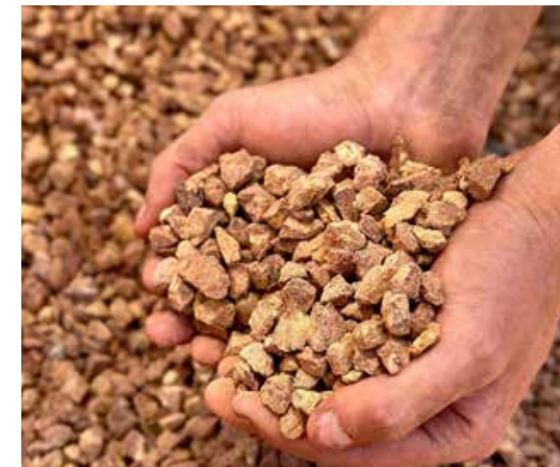
CRACKED PEA GRAVEL
