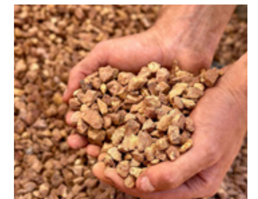
Cracked pea gravel
