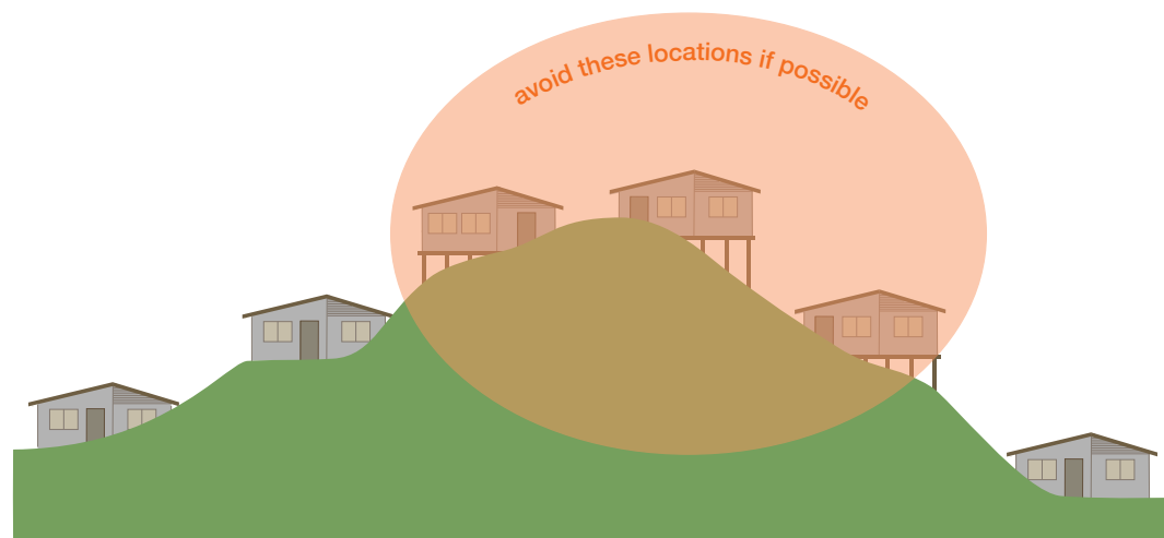
Figure 6: Topography considerations for building locations
