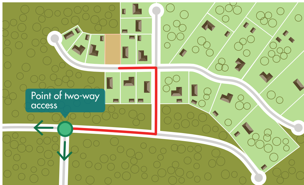
Figure 12: Demonstration of a lot achieving two-way access within 200 metres
