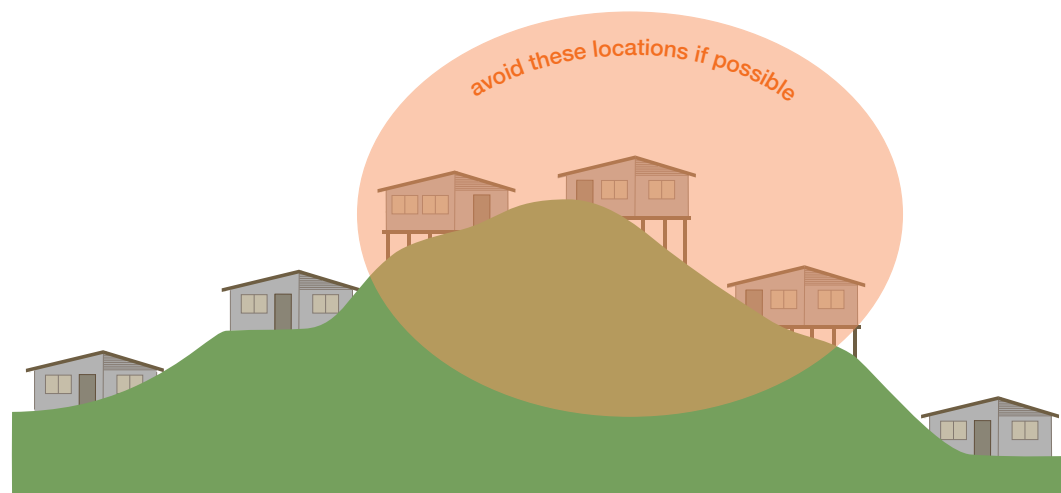
Figure 6: Topography considerations for building locations
