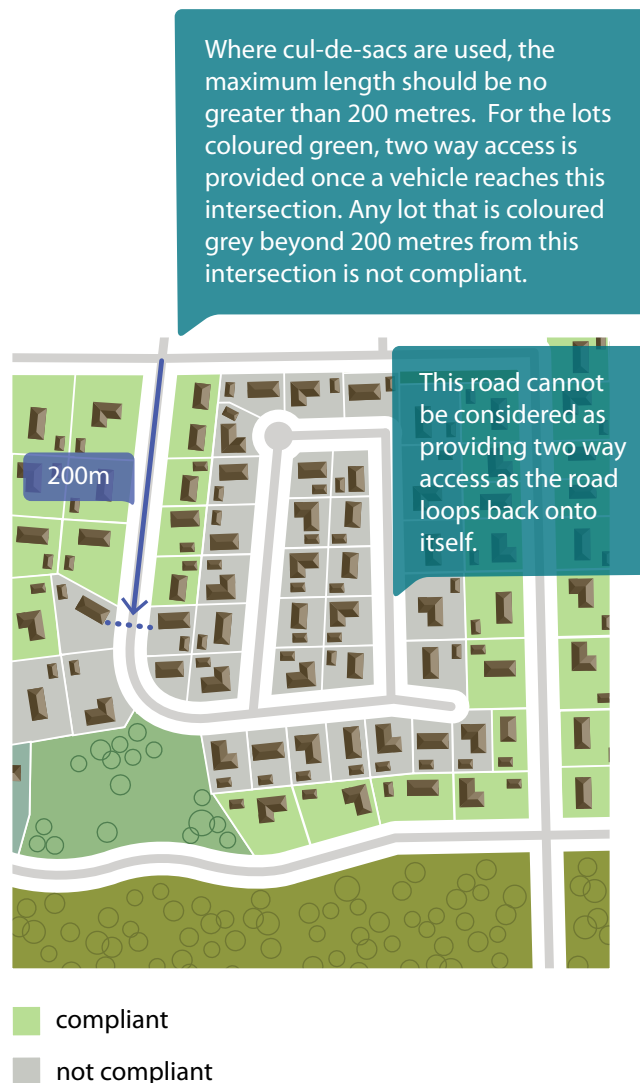
Figure 11: Example of compliant and non-compliant two-way access
