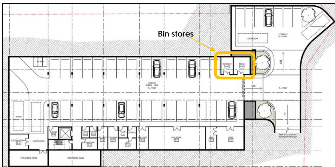
Figure 1: Basement plan showing location of bin stores
