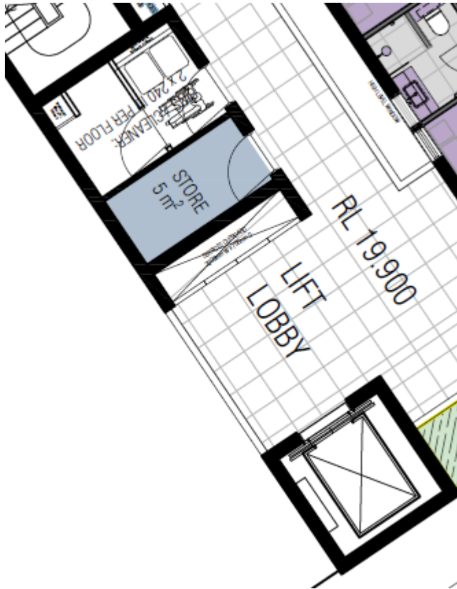
Figure 2: Individual bin rooms on each floor of each building
