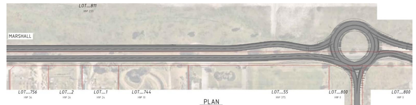
Figure 7 Marshall Road duplication 15% concept design – Beechboro Road North to Silver Swan Road – eastern section (source: City of Swan Ordinary Council Meeting, 28 July 2021 – Officers Report Item 5.1)
