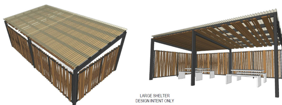
ST-01 SHELTER STRUCTURE ELEMENTS INCLUDE: STEEL FRAME CORRUGATED POLYCARBONATE ROOFING TIMBER BATTEN CLADDING TO ROOF AND SCREENING
