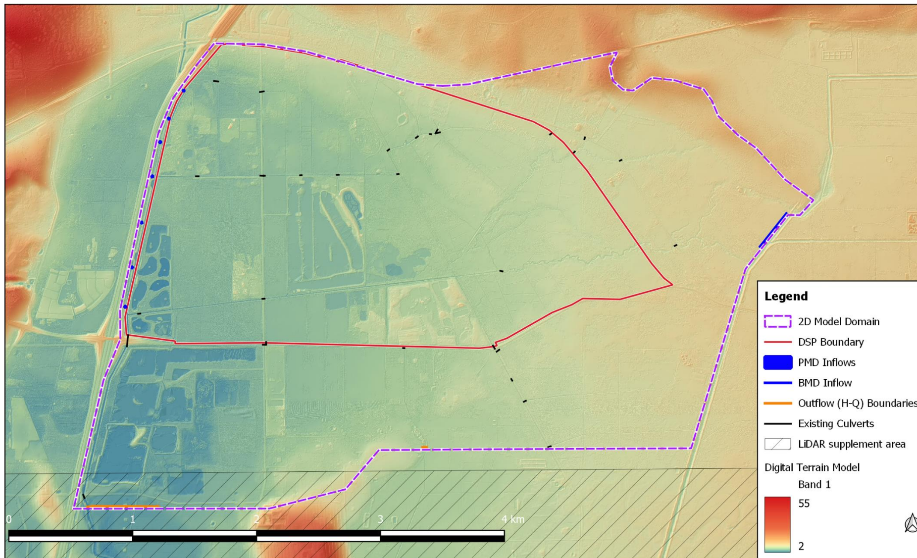
Figure 11: Existing conditions model setup and DTM
