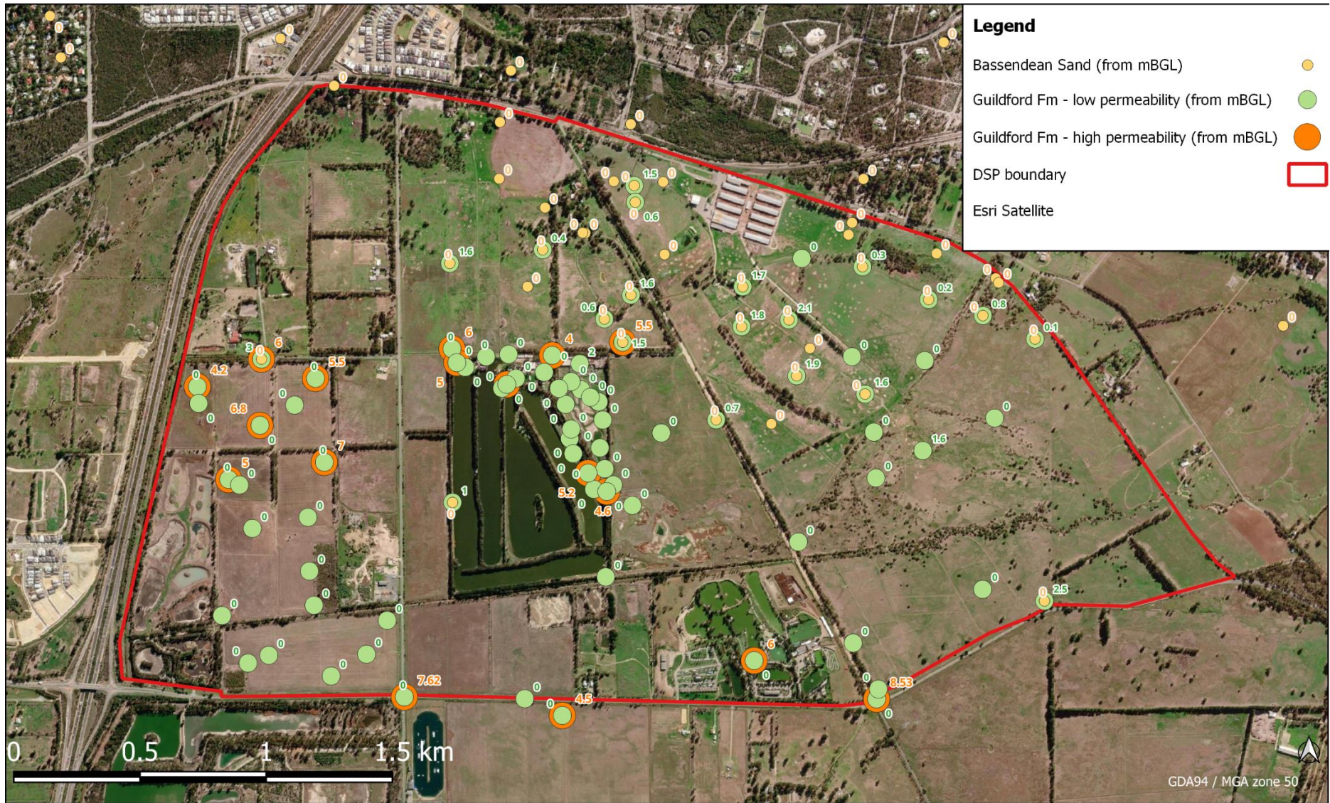
Figure 4: Depth of encountered soil types
