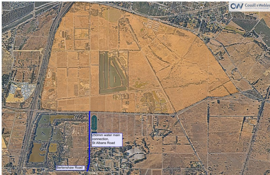
Figure 10- Water Supply Route Stage 1
