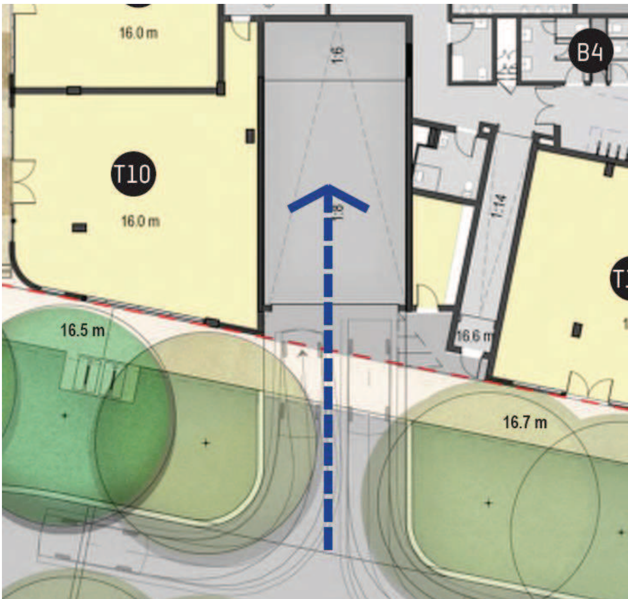
Figure 3-7 Pedestrian Ramp Gradient
