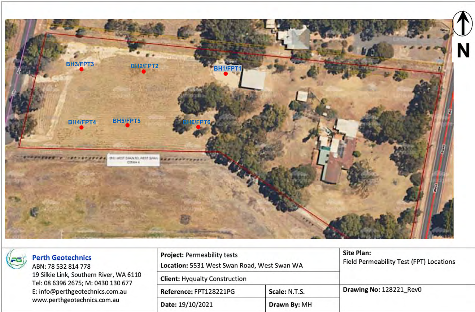
Figure 8: Soil test and permeability test holes - Perth Geotechnics (Fieldwork 14 October 2021)
