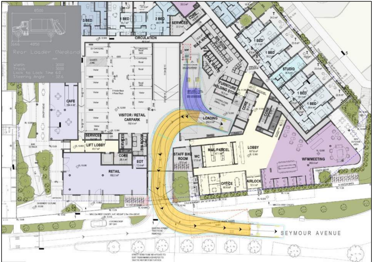
Figure 3-5 Waste Truck Swept Path – Exit
