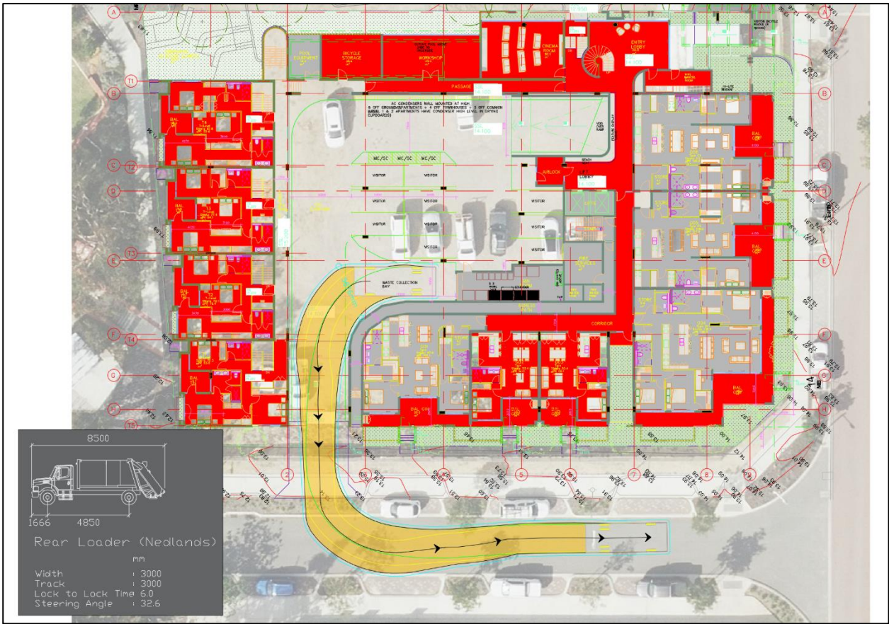
Figure 2-5 Swept Path – Waste Collection (Egress)
