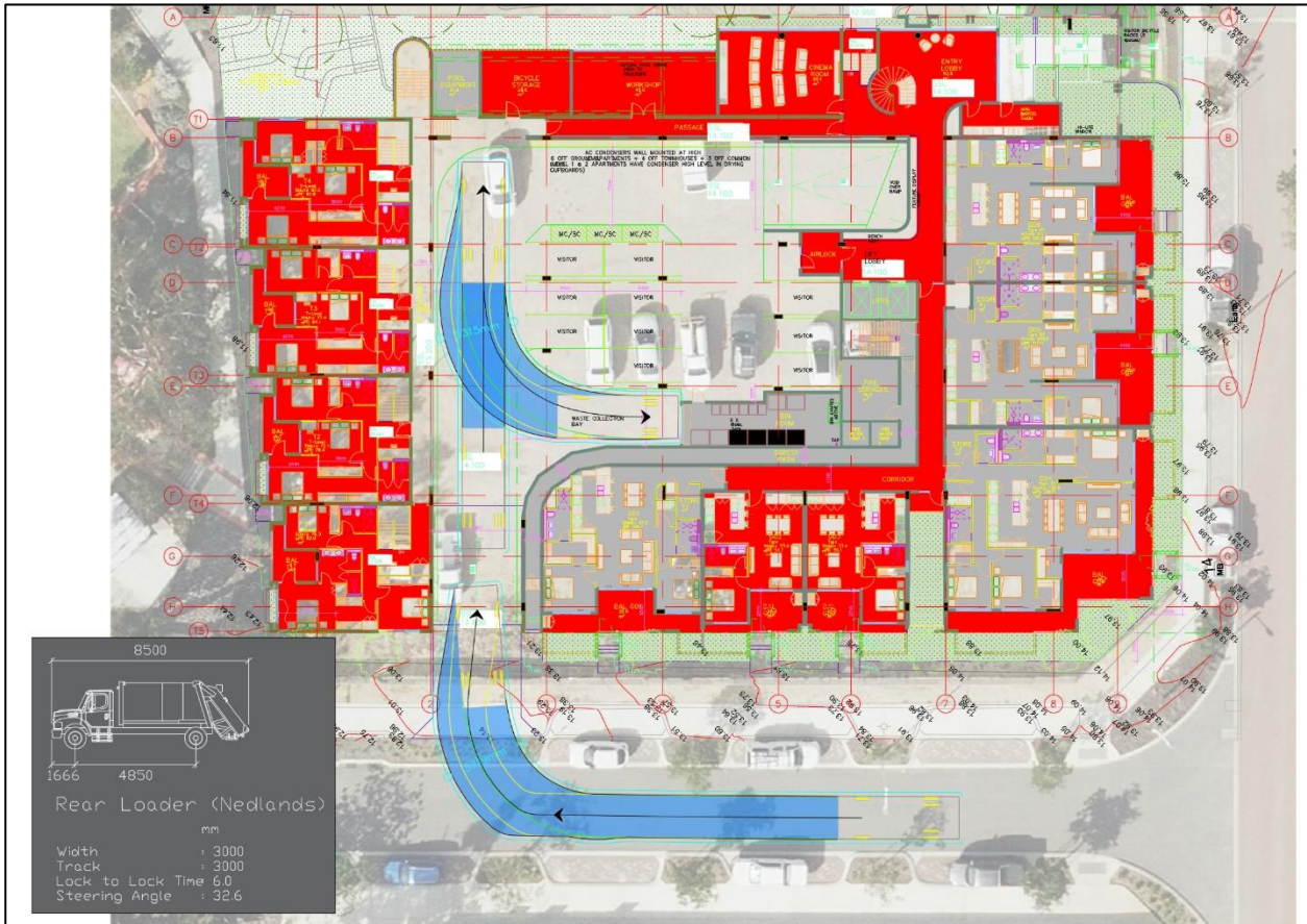
Figure 2-4 Swept Path – Waste Collection (Ingress)
