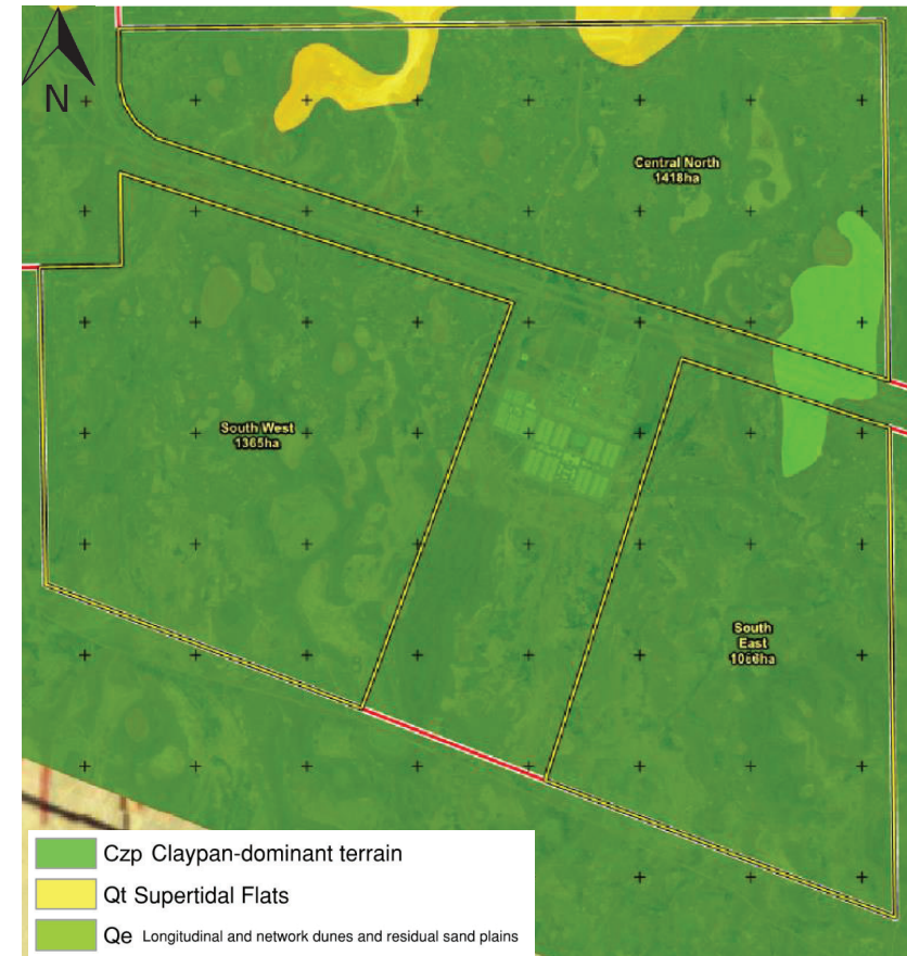
Figure 10 Geology of the ANSIA Stage 2 site (Source: Geological Survey of Western Australia, 1981)
