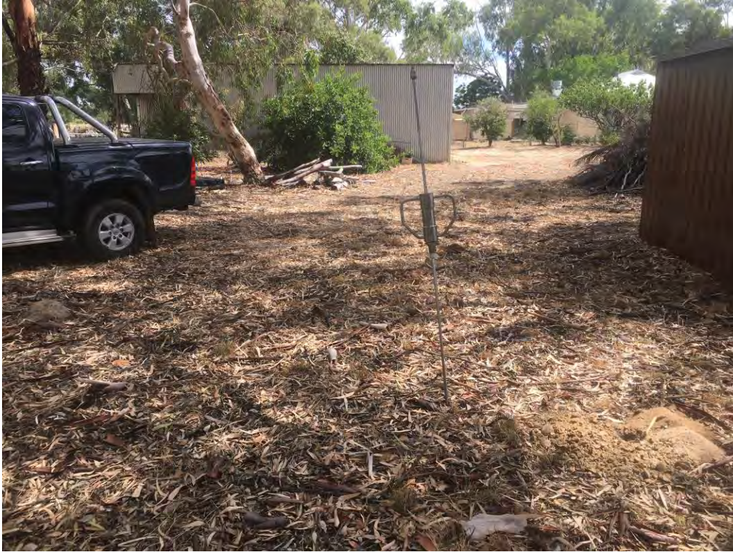
Photo 05: Conducting Dynamic Cone Penetrometer (DCP) Test at location DCP3
